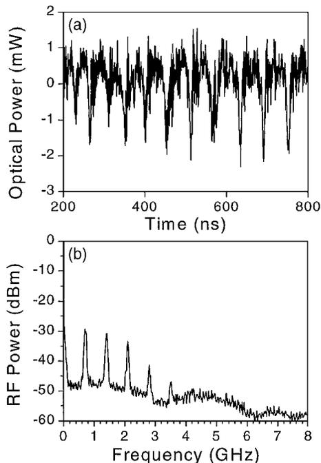
Fig. 3. LFF is observed in the absence of a second optical feedback ( $\Delta I_2 = 0$ ). (a) Fluctuations of the optical power around its average. (b) rf spectrum.
