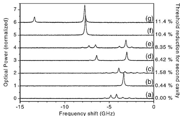
Fig. 2. Experimental optical spectra measured in double-cavity configuration as a function of threshold reduction  $\Delta I_2$  owing to the second-feedback strength. (a) LFF is observed in the absence of the second feedback. Increase of the second-feedback strength leads to stabilization [(b) and (f)] interspersed with unstable regions [(c)–(e) and (g)]. The optical spectra have been normalized with respect to the maximum of trace (b).
