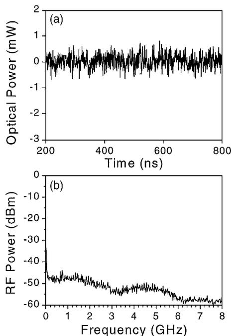
Fig. 4. Stabilization of the laser by the second optical feedback ( $\Delta I_2 = 0.44\%$ ). (a) Fluctuations of the optical power around its average. (b) rf spectrum.
