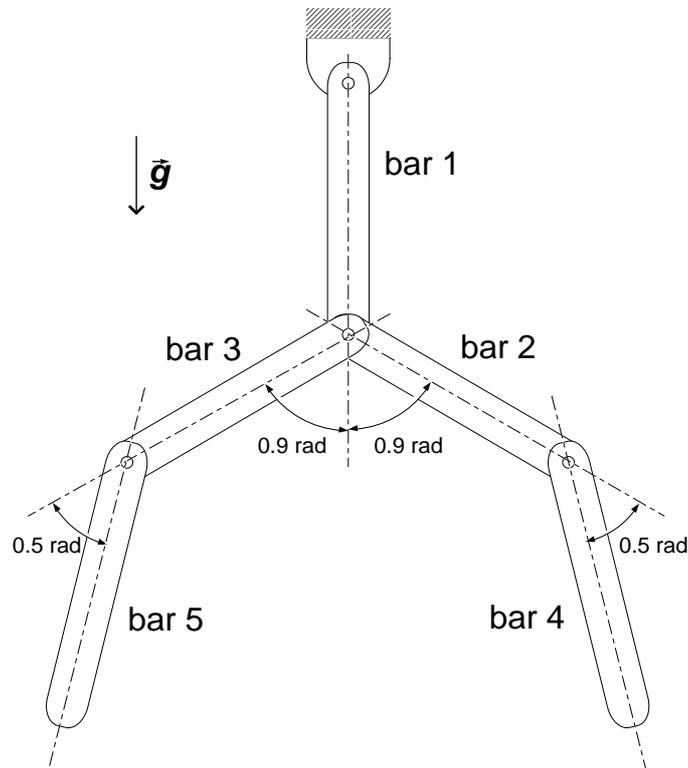
FIG. 1 – Composed pendulum with five bars
